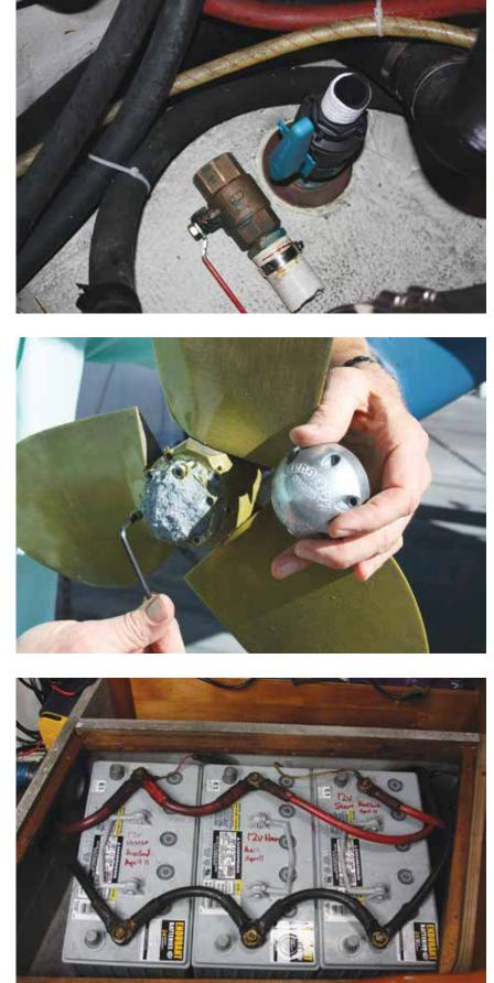
Top to bottom: replacing ball valves, changing zincs, checking batteries
