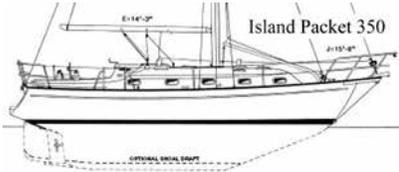
2. Modern Full Keel, with attached rudder and moderate displacement is another good choice for cruising in isolated areas where groundings or scrapes are common and the nearest shipyard may be thousands
