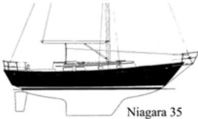
keel provides more directional stability and importantly can more easily withstand a 6 knot grounding that a narrower, higher-aspect keel. The unprotected spade rudder is more vulnerable to being damaged by groundings or hard impact
