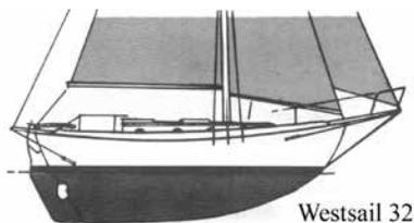
1. Heavy Displacement Full-Keeled Double-Enders based on Tahiti ketch or Norwegian lifeboat lines used to be a nearly automatic choice for long distance voyaging. However, yacht design has made great advances in the past 60 years,
