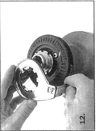
12. Re-assemble the drum, main spindle retaining collets and feeder arm. Lightly grease the 'O' ring and top cap thread before fitting.
